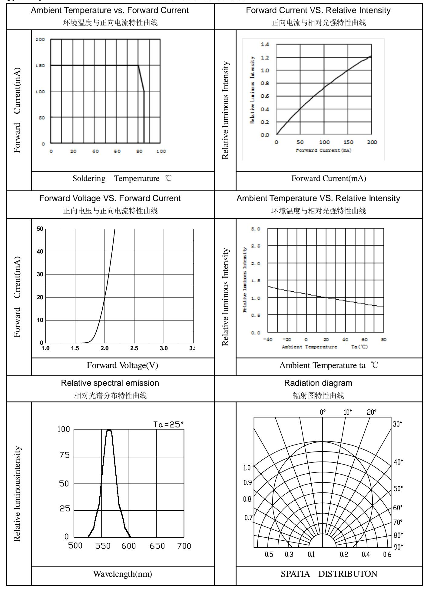
Typical optical characteristics curves 典型光学特性曲线(R)
