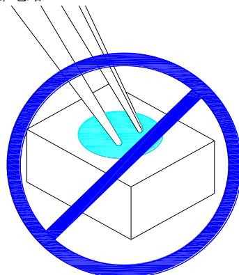
2.The outer diameter of the SMD pickup nozzle should not exceed the size of the LED to prevent air leaks. The inner diameter of the nozzle should be as large as possible. A pliable material is suggested for the nozzle tip to avoid scratching or damaging the LED surface during pickup. The dimensions of the component must be accurately programmed in the pick-and-place machine to insure precise pickup and avoid damage during production.
