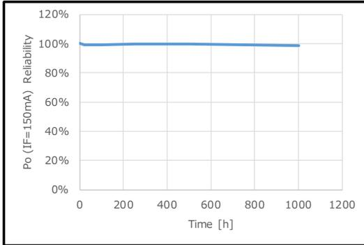
***Figure 11. 125°C Pulse 1000mA 1,000h test
