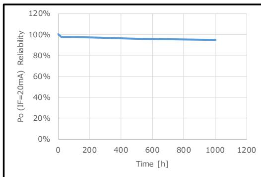
**Figure 11. 125°C 80mA 1,000h test**
