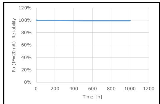
**Figure 12. 25°C Pulse 500mA 1,000h test**
