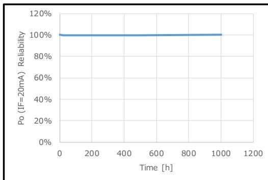
**Figure 11. 25°C Pulse 300mA 1,000h test**
