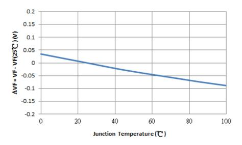
Fig.7 Delta Voltage vs Junction Temperature
