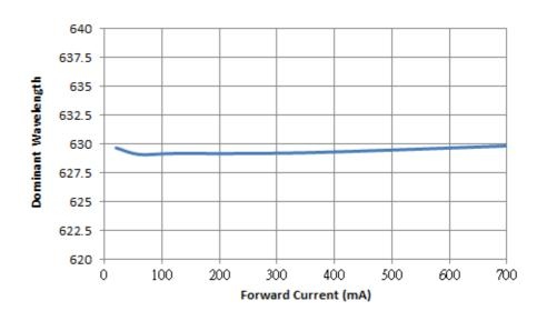
Fig.6 Dominant Wavelength vs Forward Current
