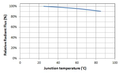
Fig.5 Relative Radiant Flux vs Junction Temperature
