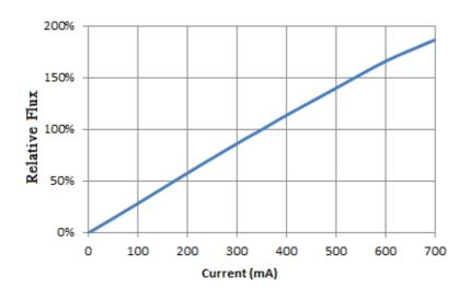
Fig 1. Relative Flux vs. Forward Current
