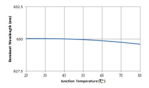
Fig.8 Dominant wavelength vs Junction Temperature
